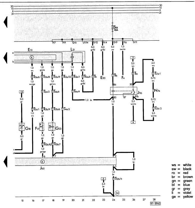
E13 - Heater-Time Temperature Control Switch, on left B-pillar, upper part
